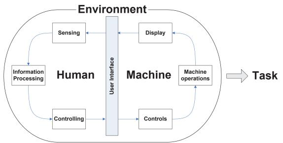
Figure 4.2 Model of a human-machine system from Chapanis (1965)
